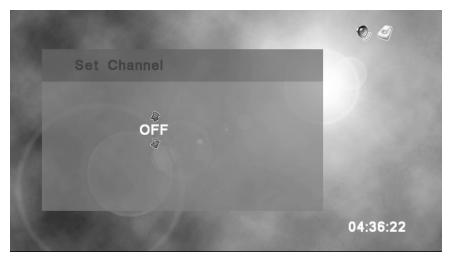
If the IR Blaster is connected and set up, you can select a specific channel (up to 4 digits). Otherwsie, you should set to OFF mode when not using an IR Blaster. Use ♦ to change each digit and ◀▶ to move between them. Once you have set the channel, press ல to complete the Recording Setup.
