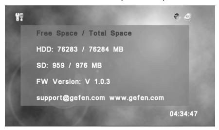
The information menu will give you statistics on the remaining and total space available on both the internal hard disk drive (HDD) and SD card.
