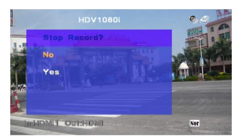
Use  $\clubsuit$  on the remote to select either Yes or No and press  $\circledcirc$ . Selecting No will continue the recording process. Selecting Yes will stop the recording process and save the movie to the currently selected media. Note that even though this dialog is displayed, the recording process is still taking place. The recording will not stop until you select Yes. NOTE: You cannot pause a recording by pressing the PAUSE button. You can only STOP a recording.
