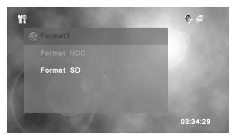
This provides you the option of formatting the internal hard disk drive (HDD) or SD Card. Warning: Formatting the internal HDD or SD Card will erase ALL data on the media!
