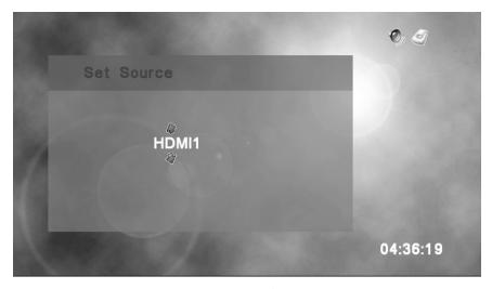
Set the input source for the recording using  $\Leftrightarrow$  to select between HDMI1, HDMI2, COMPONENT or VIDEO. Press (or) when you are done.
