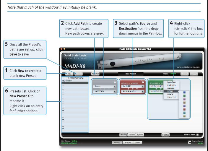
Path boxes can be locked, muted, re-coloured, cleared and deleted using the right-click drop-down menu.
