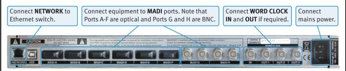
Note that X8 can either be connected directly to your computer or remotely via a wider Ethernet network. By default X8 will attempt to obtain an IP address from a DHCP server – if that fails it will fall back to a "Link Local" address. Many Ethernet networks will have a DHCP server present – most Internet (ADSL) routers for example are so equipped. See Page 9 for details of X8's hardware connections.
