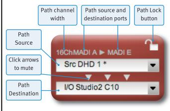
Within the Path Box, click on the upper text box (initially labelled **Source**) and select a source for the route from the drop-down list which appears.
