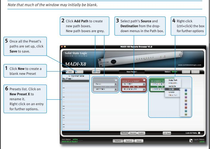
Three rows of routing boxes can be viewed at any one time, and a scrollbar appears to the right of the Preset Editor whenever there are more than 12 Path boxes. Each Path Box can contain a single route, though that route may include up to 64 channels.
