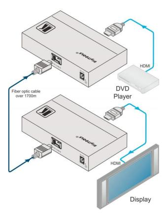
Figure 3: Connecting the 670T/670R Transmitter/Receiver System
