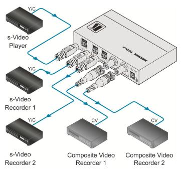
Figure 3: Connecting the 401C
