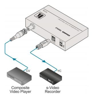
Figure 4: Connecting the 401DN
