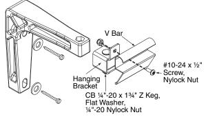
**Please note:** When installing wall brackets, flexible driver bit extensions may make it easier to accurately drive the fasteners into the mounting surface.
