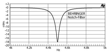
Fig. 4.1: Filter curve of a narrow-band filter
