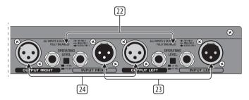
Fig. 3.6: FBQ2496's rear connections
