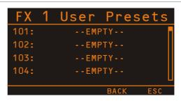
Turn the MENU/ENTER rotary encoder to select the user preset where the edited effect should be stored to. Press the MENU/ENTER rotary encoder to open the Set FX Name dialog.
