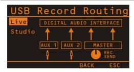
Turn the MENU/ENTER rotary encoder to select the assignment of CMS busses to channels USB 1 to 4 of the DIGITAL AUDIO INTERFACE. Following table lists the available assignments. Press the MENU/ENTER rotary encoder to apply the selected assignment. Pressing the BACK function key returns to the menu. Pressing the ESC function key discards all changes and returns to effect mode.
