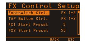
Turn the MENU/ENTER rotary encoder to highlight an entry in the left column of the FX Control Setup dialog. Press the MENU/ENTER rotary encoder to select the corresponding value in the right column. Now turn the MENU/ENTER rotary encoder to edit the value and press the MENU/ENTER rotary encoder again to apply the new
