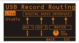
If the AUX ways are not yet reserved or occupied for monitoring, effect applications or other purposes, you can use them instead to record two additional signals, which then are available during post-production of your recording. This, for example, provides the possibility to enhance solo vocals or a solo instrument at specific passages so that they stand clearly in front of the mix. For that, you need to assign respective input channels to the AUX bus using the AUX controls. Post-fader mode is
