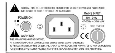
**Connecting Mains Power** Read the SAFETY INSTRUCTIONS printed at the front of this User Guide and on the rear panel. Check that the correct mains lead with moulded plug has been supplied with your console. The power supply accepts 50/60Hz AC mains voltages within the range 100-240V without changing any fuses or settings.
