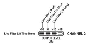
**AFS Normal vs. 6-Fixed/6-Live** - Press the **<AFS>** button on CHANNEL 2 to select through selections within menus. The selections for System Lockout are: AFS Normal Mode (All 12 filters are live) and AFS Normal vs 6-Fixed/6-Live Menu, and will be represented by a lit LED once selected. The Fixed filters stay closed until cleared, and live filters continuously update in the order that they were set. The following illustration show the selections and the corresponding LEDs indicators:
