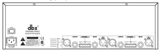
**Power Cord Receptacle:** Connects AC power to the equalizer.
