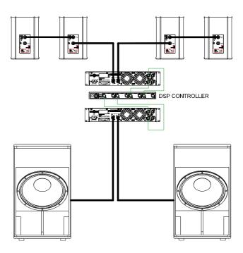
In this configuration, the frequency range of the full range system is extended in the low end.
