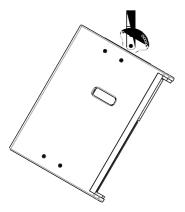
The Full Range cabinets should be located in a high position (between two or three meters), slightly inclined to the audience. If the loudspeakers are located too low, the listeners at the end of the room will not hear a good sound quality.
