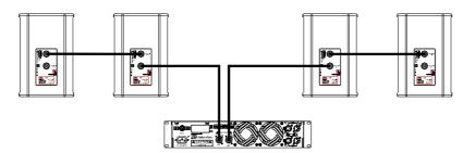
Each enclosure type is driven by the **PA Series** amplifier according the cabinet power requirements. Correct factory preset is needed.
