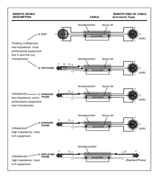
Connector and cable configurations recommended for use with the CPR-series. These cables are based on the use of auxiliary equipment that is isolated from the AC power mains.
