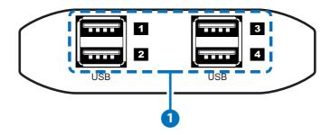
1 USB 1~4: Use to connect to USB devices such as flash drives, external HDDs, digital cameras, printers, and etc.
