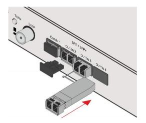
Figure 4: Installing the SFP Modules
