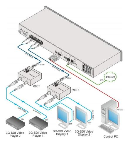
Figure 3: Connecting the VS-44FO
