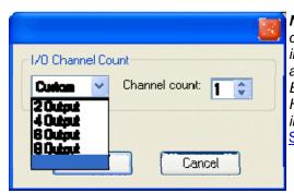
**Note:** CobraNet Output blocks of less than 8 channels may now be used. When a block is placed into the Layout from the Object Toolbar, a dialog will appear, allowing the Channel Count to be specified. Each block must still have a unique bundle number. However, smaller Channel Counts will allow for an increase in the use of 'flexible CobraNet bundles' (see System Network Considerations).
