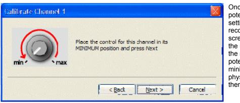
Once the maximum potentiometer setting has been recorded, this screen will prompt the user to adjust the same potentiometer to its minimum (lowest) physical setting, then select "Next".
