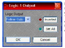
Logic Outputs affects individual Logic Output settings, but may be applied to all Logic Outputs. (Logic Outputs must be designated when placing Auto Mixers from the Object Toolbar). Logic Output selects Follow Gate, On, or Off condition of the Logic Output. Invert reverses operation of the Logic Output (off when channel active). Set All causes current Logic Output settings to be applied to all channels.
