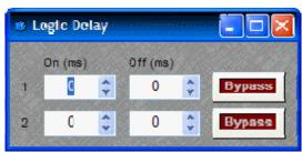
Logic Delays are connected between the output and input control nodes of other components in the layout. These other components may represent internal or external control functions. When a change (on/off) occurs at the Logic Delay input, and remains in that condition beyond the designated delay time, the Logic Delay output will then produce that same change.
