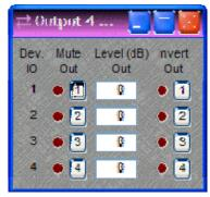
**Device IO** indicates which hardware output is associated with that software channel. **Mute Out** turns the output signal on/off. **Level Out** adjusts the relative output volume. **Invert Out** reverses the polarity of the output signal.
