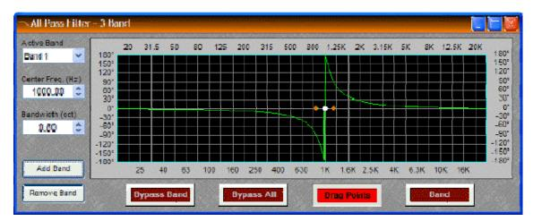
All-Pass Filters are so named because they do not affect frequency response. Instead, they affect signal phase only and, therefore, can be used to compensate for the phase anomalies caused by normal equalization filters. All-Pass Filters are available with up to sixteen bands.
