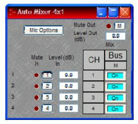
**Mute In** turns the input signal on/off. **Level In** adjusts the relative input volume. **Ch / Bus** assigns inputs to the output. **Mute Out** turns the output signal on/off. **Level Out** adjusts the relative output volume.
