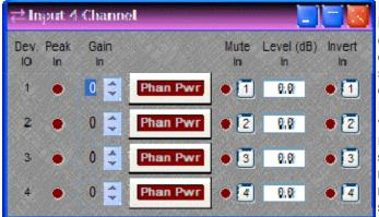
**Device IO** indicates which hardware input is associated with that software channel. **Gain In** compensates for different input levels (mic or line), and should be set so **Peak In** flashes only occasionally (6dB headroom). **Phan Pwr** assigns +48 Volt phantom power to the input for condenser microphones. **Mute In** turns the input signal on/off. **Level In** adjusts the relative input volume. **Invert In** reverses the polarity of the input signal.
