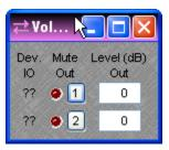
Double-clicking the Transmit block produces a control dialog box with settings for level adjustment and muting of outgoing audio signals.
