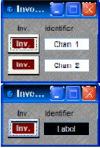
**Invert** reverses the polarity of the audio signal (180°). **Identifier** provides a custom label, when the dialog box is minimized (see below).
