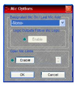
**Designated Mic On / Last Mic Hold** determines which microphone (if any) will stay/become active when no signal is present. **Logic Outputs Follow Mic Logic** assigns logic outputs to follow Designated Mic On / Last Mic Hold. **Open Mic Limits** enables (and designates) a maximum allowable number of active microphones.
