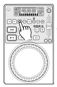
Figure 9: Tapping the reverse track button will jump back to the previous track.
