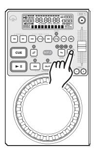
**Using the PITCH SLIDER (5):** Be sure the pitch function has been activated as described above. To use the *PITCH SLIDER (5)* slide the slider up and down. Down will increase the pitch and up will decrease the pitch.
