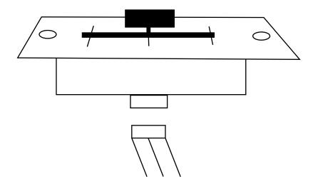
The crossfader is "Hot Swapable" which means it may be replaced at any time, even when power is applied. Only replace with American Audio Part Feather Fader Plus. Replacing with any other model fader may seriously damage your mixer. Please, always use insulated tools.
