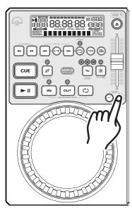
Holding down or tapping on the (-) PITCH BEND BUTTON (8) will provide a slow down in the playback pitch.
