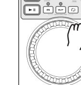
Holding down or tapping on the (+) PITCH BEND BUTTON (8) will provide a speed bump in the playback pitch.
