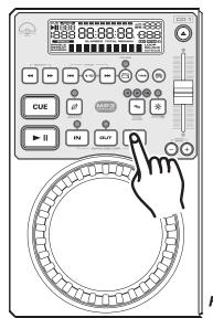
**REPLAY LOOP** - The RELOOP function allows you to return to your stored loop at any time. The *IN BUTTON (10)* and *OUT BUTTON (10)* LEDs will indicate a loop is stored in memory, and may be played at any time. To replay the loop, press the *RELOOP BUTTON (10)*. The *IN BUTTON (10)* and *OUT BUTTON (10)* LEDs will again begin to flash indicating SEAMLESS LOOP mode has been activated and your loop will immediately begin to play.
