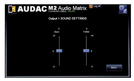
This screen shows two faders. One to control the bass (low tones) which can be adjusted from -9 to 9 dB. The other controls the treble (high tones) and can also be adjusted from -9 to 9 dB.
