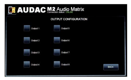
Now a new screen appears which allows you to change the settings of this output. Following options can be adjusted or applied: set volume, apply several different filters, apply a 3 or 7 band equalizer, set quick menu settings, set output linking settings and set talkover settings by clicking the corresponding button. Also the output can be toggled between mono and stereo or toggle between Single—ended and Balanced. Even antiphase and a delay time can be set for a certain output.
