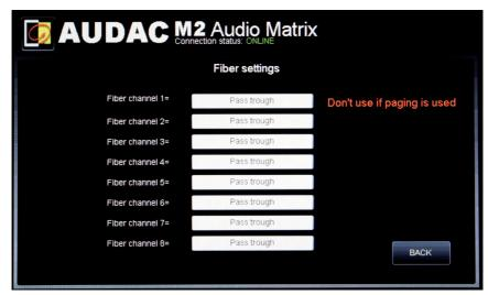
For every of the eight fiber channels you can set an input to link with other M2 or R2 units or pass through to take an input from a M2 or R2 unit and pass it through to an other M2 or R2 unit.
