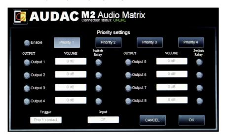
To do a priority setting first choose a channel on which the M2 will trigger your setting. Now an input should be chosen. You can select every output to which the input should be routed. For every output it is possible to set volume and toggle relay position.
