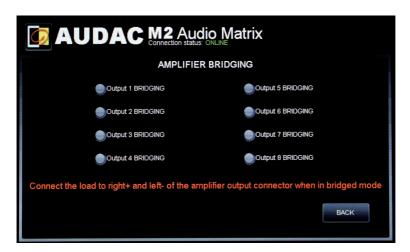
Select the output channels you want to bridge. Bridging an output will result in a mono output with double power.
