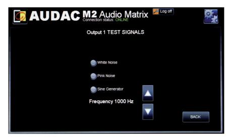
When one of the test signals is selected, "Other" will appear in the 'Input Selection" box on the main screen.
