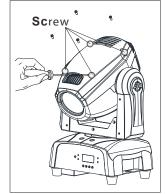
4. Unscrew the 4 screws located on the other side
