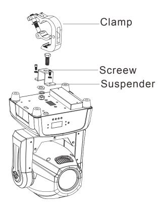
Screw one clamp via a M12 screw and nut to the included bracket. Attach the bracket using the omega locks to the bottom of the Focus Spot Two. Attach and pull the safety-cable through one of the safety holes located on the bottom base and over the trussing system or a safe fixation spot. Insert the end in the carabine and tighten the safety screw.
